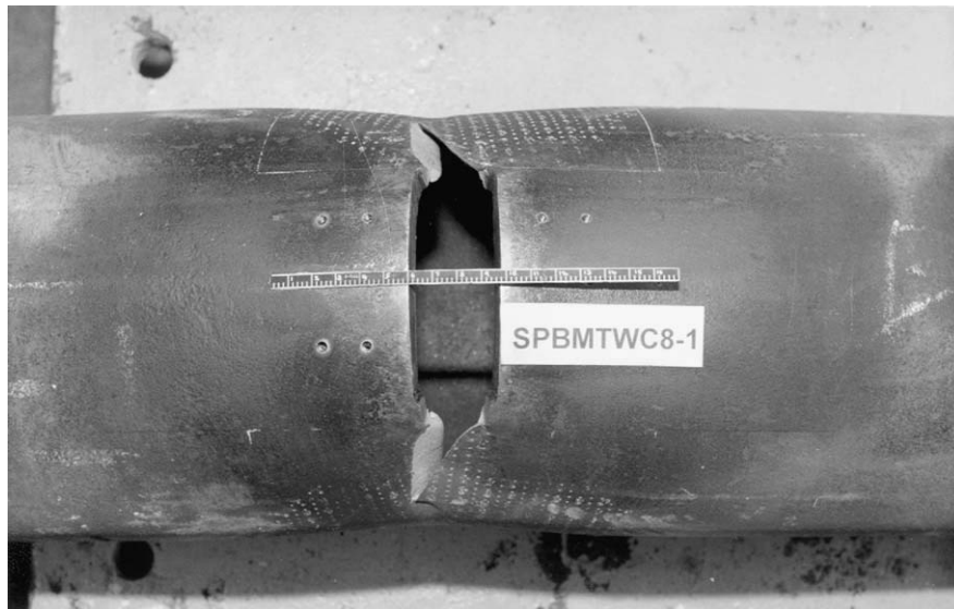
Fig. 5. Typical crack growth pattern in pipe test specimen no. SPBMTWC8-1.
